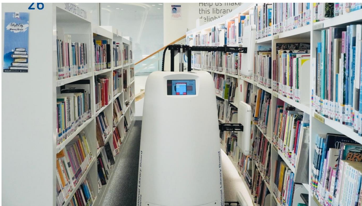
Fig. 4 – Shelf Reading Robot in action of scanning shelves with its multiple arms.
