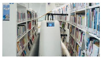
Figure 4. Shelf Reading Robot in action of scanning shelves with its multiple arms.
